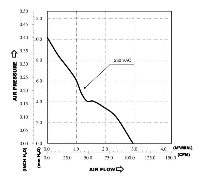
\*TEST CONDITION: INPUT VOLTAGE-----OPERATION VOLTAGE
