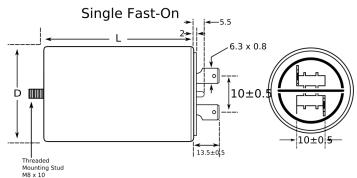
Dielectric Film/Foil Polypropylene Style Plastic Case and Cover, Ultra Sonically Welded Description Ultra Sonically Welded Seal, Safety Class PO, Features UL 94 V0 Disk **RoHS** Yes Lead Fast On (1+1) UL, VDE, UL (Construction Only), UL\_94 VO Qualifications Disk AEC-Q200 No Component 26 g Weight
