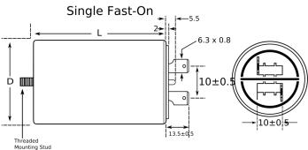
Ultra Sonically Welded Seal, Safety Class PO, Features UL 94 V0 Disk **RoHS** Yes Lead Fast On (1+1) UL, VDE, UL (Construction Only), UL\_94 VO Qualifications Disk Mounting Stud M8 x 10 AEC-Q200 No Component 26 g Weight
