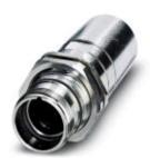
Rear panel feed-through, straight, Screw locking, M23, Axial O-ring, Central fixing, shielded: yes, cable diameter range: 6.5 mm ... 14.5 mm
