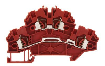
Double-level terminal, Tension-spring connection, Mounting type: Mounting rail TS 35/7.5, Rated cross-section: 2.5 mm², Width: 5.1 mm, Colour: Red
