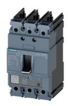
circuit breaker 3VA5 UL frame 125 breaking capacity class H 65kA @ 480V 3-pole, line protection TM230, FTAM, In=125A overload protection Ir=125A fixed short-circuit protection Ii=5...10 x In UL 489 SB (naval), 50° C without connection
