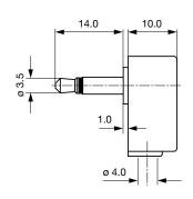
Cable diameter max. 4.0 mm
