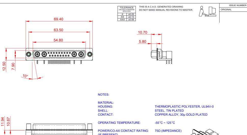
(IF PRESENT) SIGNAL CONTACT CURRENT RATING: 5A PER CONTACT SIGNAL CONTACT RESISTANCE: 10mΩ MAX.
