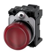
Indicator lights, 22 mm, round, plastic, red, lens, smooth, with holder, LED module with integrated LED 110 V AC, spring-type terminal, with laser labeling, inscription or symbol Customer-specific selection with SIRIUS ACT configurator (CIN)
