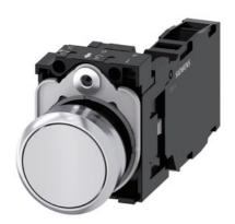
Pushbutton, 22 mm, round, metal, shiny, white, pushbutton, flat, momentary contact type, with holder, 1 NO+1 NC, screw terminal, with laser labeling, symbol number according to, ISO 7000 or IEC 60417
