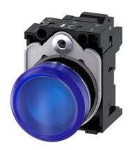
Indicator lights, 22 mm, round, metal, shiny, blue, lens, smooth, with holder, LED module with integrated LED 110 V AC, spring-type terminal, with laser labeling, symbol number according to, ISO 7000 or IEC 60417
