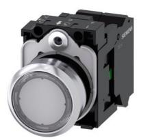
Illuminated pushbutton, 22 mm, round, metal, shiny, clear, pushbutton, flat, momentary contact type, with holder, 1NO, LED module with integrated LED 110 V AC, spring-type terminal, with laser labeling, symbol number according to, ISO 7000 or IEC 60417
