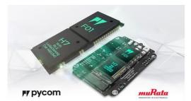
Above is the F01 H7 with the m.2 donor board mounted on our new Expansion Board.
