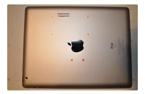
If you're happy with how the marks look, go ahead and drill 'em! The two large holes are #3 Metric, and the smaller ones are for the #2. Be careful not to overdrill the holes.
