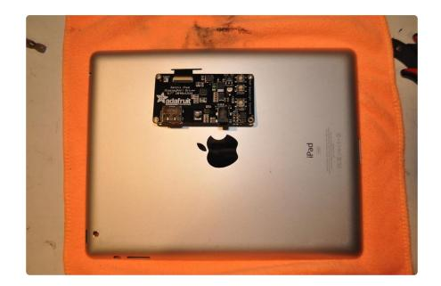
Now, use your fine tipped marker to mark where the mounting holes line up. Another method is to place the board on an 8x11 sheet of paper, and create a drilling stencil. Then, hold the back panel up to the head of your lamp, and mark where you need to drill the holes for the lamp mount. The ideal place for the lamp is not dead center, but slightly offset towards the side with the rear facing camera.
