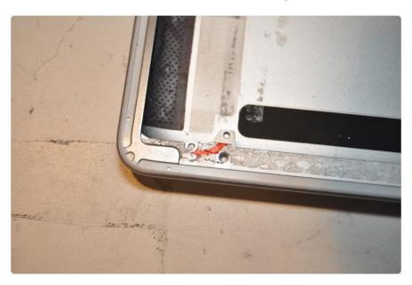
Next, place the screen into the back panel, and observe where the ribbon cable will need to exit the case. You will need to make a cut with your Dremel to pass this cable through the case, and out to the Qualia board.
