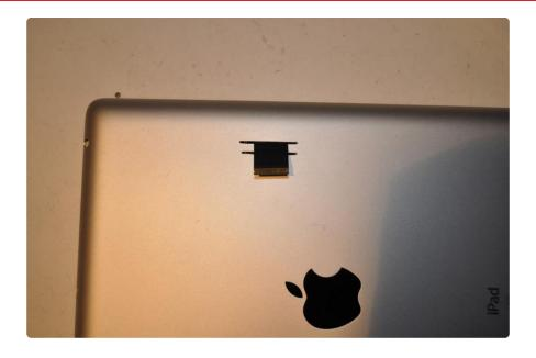
Using the ribbon as your guide, place your Qualia bareboard where you should mount it on the back of the iPad back panel. The ribbon should not flex or bend in a strange way. Try to align it so that it goes straight into the Qualia.
