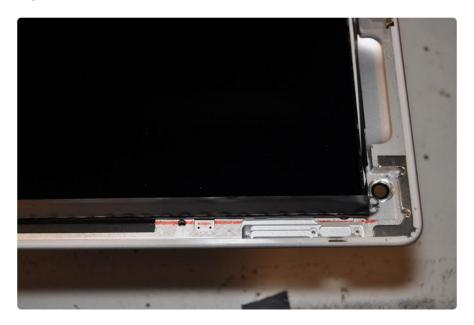
For the corner on the same side, but closer to the dock connector, a small section must be ground down. You should not cut this piece competely off, as it will be good to have support underneath the Retina Display's mounting bracket. You should shave a millimeter or two down. The area is marked with orange marker here.
