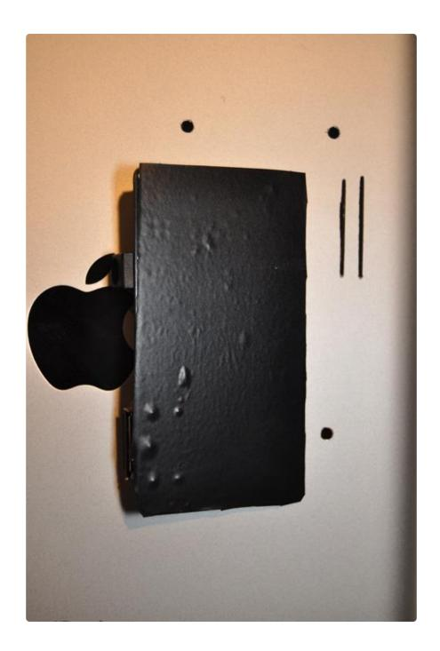
Okay, you're ready to attach the Qualia! Put a 2x8mm screw through each of the holes for the Qualia in the back panel, with the heads on the inside of the iPad. Place a #2 plastic washer on each of the machine screws. Now, drop the Qualia board onto the screws, and secure it with the #2 metric hex nuts.
