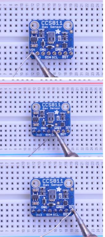
Add the breakout board and Solder: Place the breakout board over the pins so that the short pins poke through the breakout pads
