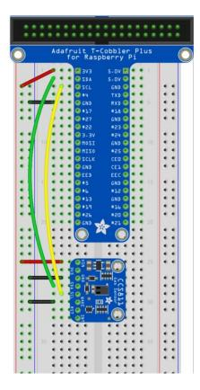
Now you should be able to verify that the sensor is wired up correctly by asking the Pi to detect what addresses it can see on the I2C bus:
