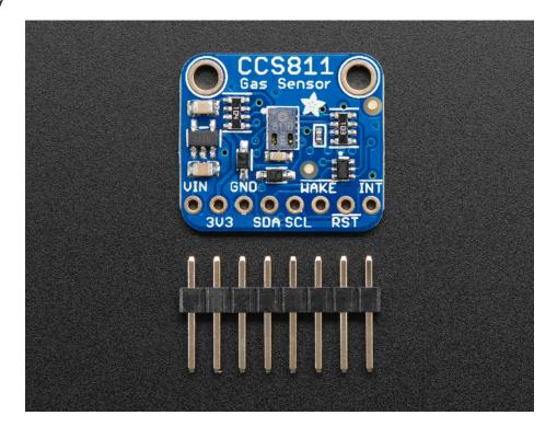
Before use, you'll need to attach headers so you can plug in this sensor into a breadboard. Soldering is essential!
