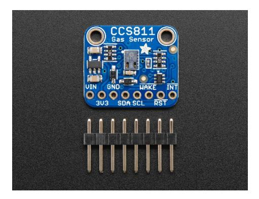
The CCS811 has a configurable interrupt pin that can fire when a conversion is ready and/or when a reading crosses a user-settable threshold. The CCS811 supports multiple drive modes to take a measurement every 1 second, every 10 seconds, every 60 seconds, or every 250 milliseconds.
