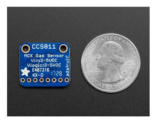
The CCS811 has a 'standard' hot-plate MOX sensor, as well as a small microcontroller that controls power to the plate, reads the analog voltage, and provides an I2C interface to read from.
