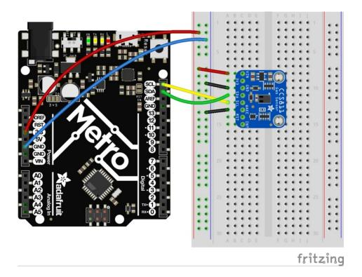
Don't forget to tie WAKE to Ground - this is required!
