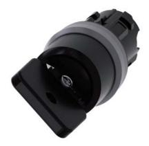
Key-operated switch O.M.R, 22 mm, round, plastic with metal front ring, lock number 73034, black, with 2 keys, 2 switch positions O-I, latching, actuating angle 90°, 10:30h/13:30h, key removal O, with laser labeling, upper case and lower case, always upper case at the beginning of the word
