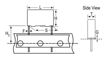
General Information Series Dielectric Metallized Polypropylene Style Radial Features MKP EMI Safety RoHS Lead Wire Leads Safety Class X1 Qualifications ENEC, UL, cUL, CQC AEC-Q200 No THB Performance No 2.961 g Component Weight Miscellaneous ClimCat: 40/110/56/B Shelf Life 104 Weeks
