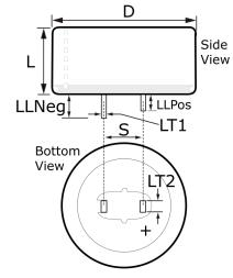
General InformationSeriesFYHDescriptionRadial Cylindrical Double Layer CapacitorRoHSYesAEC-Q200NoComponent Weight2.2 gMiscellaneousDischargeValue = 0.075 F.
