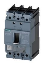
circuit breaker 3VA5 UL frame 125 3-pole, starter protection TM120M, AM, In=2A without overload protection short-circuit protection Ii=3...7 x In nut keeper kit on both sides
