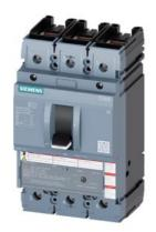
circuit breaker 3VA5 UL frame 250 breaking capacity class H 65kA @ 480 V 3-pole, line protection TM230, FTAM, In=175A overload protection Ir=175A fixed short-circuit protection Ii=5...10 x In UL489 SB (naval), 50 deg. cel. cable connection on both sides
