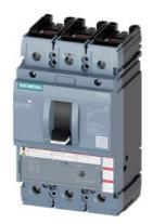
circuit breaker 3VA5 UL frame 250 3-pole, starter protection TM120M, AM, In=200A without overload protection short-circuit protection li=3...6 x In cable connection on both sides
