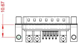
75Ω (IMPEDANCE) POWER/CO-AX CONTACT RATING: (IF PRESENT) SIGNAL CONTACT CURRENT RATING: 5A PER CONTACT SIGNAL CONTACT RESISTANCE:  $10m\Omega$  MAX. INSULATOR RESISTANCE:
