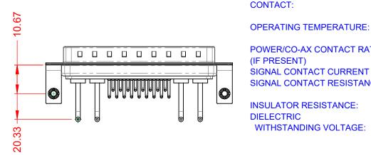
10A (CURRENT) POWER/CO-AX CONTACT RATING: (IF PRESENT) SIGNAL CONTACT CURRENT RATING: 5A PER CONTACT SIGNAL CONTACT RESISTANCE:  $10m\Omega$  MAX. **INSULATOR RESISTANCE:** 5000MΩ min. DIELECTRIC
