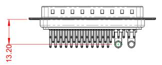
POWER/CO-AX CONTACT RATING:40A (CURRENT)(IF PRESENT)SIGNAL CONTACT CURRENT RATING:5A PER CONTACTSIGNAL CONTACT RESISTANCE:10mΩ MAX.INSULATOR RESISTANCE:5000MΩ min.DIELECTRIC5000MΩ min.
