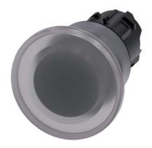
Illuminated mushroom pushbutton, 22 mm, round, plastic with metal front ring, clear, 40 mm, momentary contact type, with laser labeling, inscription or symbol Customer-specific selection with SIRIUS ACT configurator (CIN)
