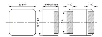
Series MPX Style SMD Chip Size 2213(9088) Description Surface Mount Inductor Features Power Inductors **RoHS** Yes Core Composite Miscellaneous 40 (K) Temperature Rise Max.
