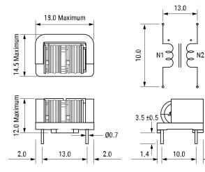
SeriesSSRH7H-MStyleThrough-HoleRoHSYesNotesM05 Lot No.MiscellaneousTemperature Rise Maximum: 55 K.CoreMn-Zn Ferrite
