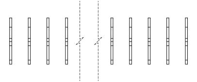
NOTE: **CONTACTS ARE HELD IN** A CARRIER FOR EASE OF ASSEMBLY
