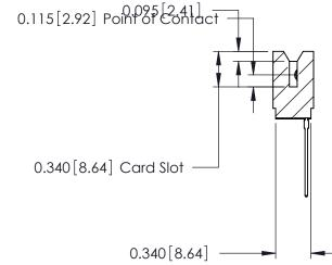
ACAD REFERENCE NO. 746 Series Ultra-Mate Card Edge Connector - Press Fit DRAWN: J.LEE Part Number: 746-028-541-506 CHECKED: **EDAC INC** SCALE: THESE DRAWINGS AND SPECIFICATIONS ARE THE PROPERTY OF EDAC INC.,AND TORONTO, ONTARIO SHALL NOT BE REPRODUCED, OR COPIED DRAWING NUMBER CANADA OR USED AS THE BASIS FOR THE 746-ENG MASTER MANUFACTURE OR SALE OF APPARATUS YOUR CONNECTION TO QUALITY & SERVICE WITHOUT WRITTEN PERMISSION.
