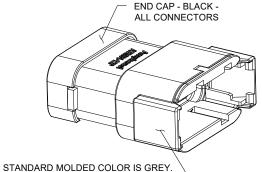
12 POS, RECEPTACLE, PIN, KEYED, ATM SERIES, SNAP FIT
