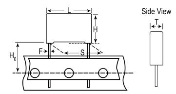
**General Information** Series R46 275 VAC Dielectric Metallized Polypropylene Style Radial EMI Safety Features RoHS Yes Lead Wire Leads Safety Class X2 ENEC, UL, cUL, CQC Qualifications AEC-Q200 No **THB** Performance No **Component Weight** 1.122 g We Recommended To Use R46 @ 310 VAC. Notes
