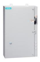
Non-reversing motor starter Size 2 1/2 Three phase full voltage Solid-state overload relay OLRelay amp range 25-100A Combination type 100A non-fusible disconnect Encl NEMA type 4X 316 S-steel Water/dust tight non-corrosive Standard width enclosure
