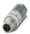
Connector, Universal, 5-position, shielded, Plug straight M12, A-coded, Crimp connection, knurl material: Zinc die-cast, nickel-plated, external cable diameter 4.5 mm ... 7.5 mm, without crimp contacts
