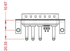
POWER/CO-AX CONTACT RATING: (IF PRESENT) SIGNAL CONTACT CURRENT RATING: 5A PER CONTACT
