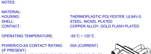
SIGNAL CONTACT CURRENT RATING: 5A PER CONTACT SIGNAL CONTACT RESISTANCE: 10mΩ MAX.
