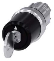
key-operated switch Siemens, 22 mm, round, metal, shiny, lock number SSG10, with 2 keys, 3 switch positions I>O<II, momentary contact type, actuating angle  $2x45^{\circ}$ , 10:30h/12h/13:30h, key removal O, with laser labeling, upper case and lower case, always upper case at the beginning of the word
