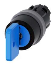
Key-operated switch O.M.R, 22 mm, round, plastic with metal front ring, lock number 73038, blue, with 2 keys, 3 switch positions I-O<II, left latching, right momentary contact type, actuating angle 2x45°, 10:30h/12h/13:30h, Key removal O Z=50-unit packaging
