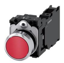
Pushbutton, 22 mm, round, metal, shiny, red, pushbutton, flat, momentary contact type, with holder, 1 NO+1 NC, spring-type terminal, with laser labeling, inscription or symbol Customer-specific selection with SIRIUS ACT configurator (CIN)
