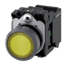
Illuminated pushbutton, 22 mm, round, plastic with metal front ring, yellow, pushbutton, flat, momentary contact type, with holder, 1NO, LED module with integrated LED 24 V AC/DC, spring-type terminal, with laser labeling, inscription or symbol Customer-specific selection with SIRIUS ACT configurator (CIN)
