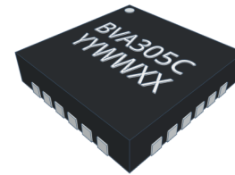
24-lead 4mm x 4mm x 0.9mm QFN
