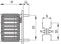
General InformationSeriesSC-JHStyleThrough-HoleRoHSYesNotesLead Spacing (S/S1) Are For Reference Only.MiscellaneousTemperature Rise Maximum: 78 K.CoreMn-Zn Ferrite
