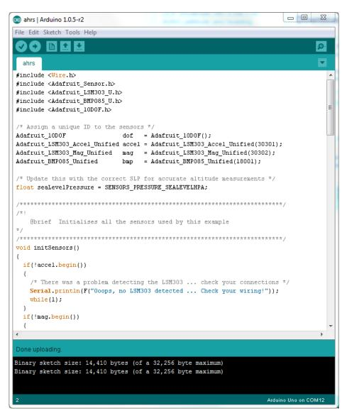
If you compile the sketch and then program your Uno with the code, you should be able to open up the **Serial Monitor** (Tools > Serial Monitor), set the baud rate to 115200, and see the following output:
