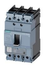
circuit breaker 3VA5 UL frame 125 breaking capacity class H 65kA @ 480 V 3-pole, line protection TM230, FTAM, In=125A overload protection Ir=125A fixed short-circuit protection Ii=5...10 x In UL489 SB (naval), 50 deg. cel. cable connection on both sides
