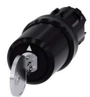
Key-operated switch BKS, 22 mm, round, plastic, lock number S1, with 2 keys, 3 switch positions I-O-II, latching, actuating angle 2x45°, 10:30h/12h/13:30h, Key removal II, with laser labeling, upper case and lower case, always upper case at beginning of line
