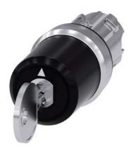
key-operated switch Siemens, 22 mm, round, metal, shiny, lock number SSG10, with 2 keys, 3 switch positions I>O<II, momentary contact type, actuating angle 2x45°, 10:30h/12h/13:30h, key removal O, with laser labeling, inscription or symbol customer-specific selection with SIRIUS ACT configurator (CIN)
