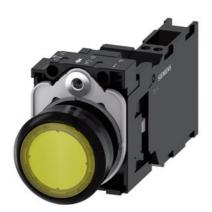
Illuminated pushbutton, 22 mm, round, plastic, yellow, pushbutton, flat, momentary contact type, with holder, 1 NO+1 NC, LED module with integrated LED 24 V AC/DC, spring-type terminal, with laser labeling, inscription or symbol Customer-specific selection with SIRIUS ACT configurator (CIN)
