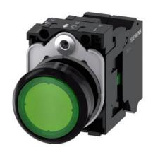
Illuminated pushbutton, 22 mm, round, plastic, green, pushbutton, flat, momentary contact type, with holder, 1NO, LED module with integrated LED 24 V AC/DC, spring-type terminal, with laser labeling, upper case
