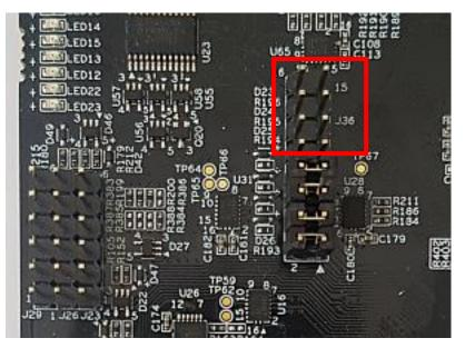
The default jumper position is to have jumpers inserted in each position of J36 which will connect the UART directly to be used by the Bluetooth interface of the M.2 connector. This behaviour prevents the UART tests described in this chapter so while testing make sure that there are no jumpers inserted in the top four positions in J36.
