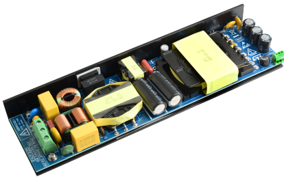
EVL012LED: 200W Wide input range LED driver
