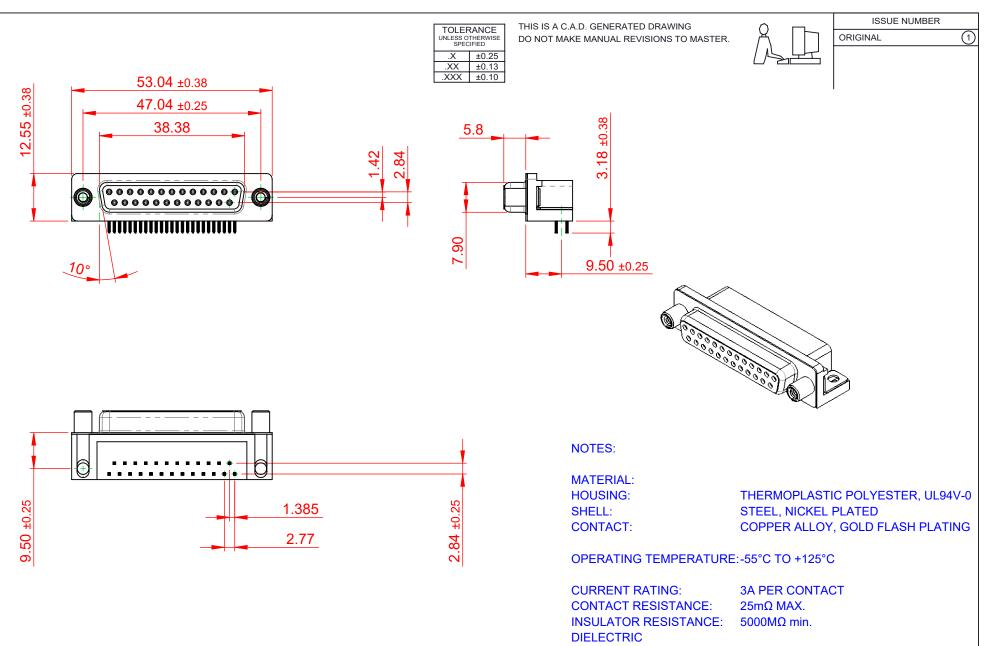
WITHSTANDING VOLTAGE: 1000V AC rms
